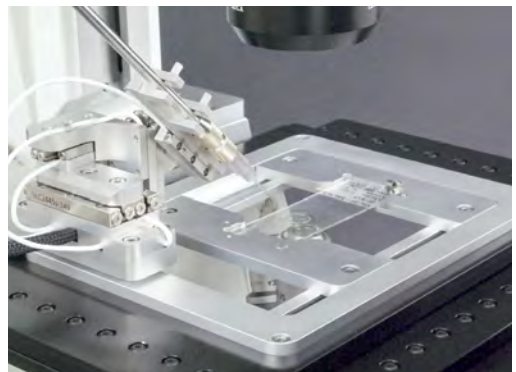
A customized four-axis micro-manipulator allows positioning of tools with nanometer precision in front of the objective lens.
